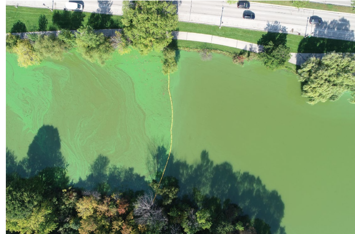
W – View of Turbidity Curtain
