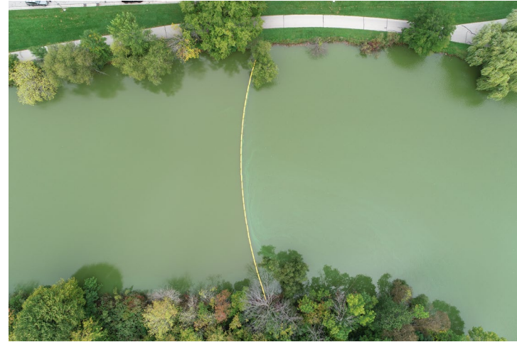
W – View of Turbidity Curtain
