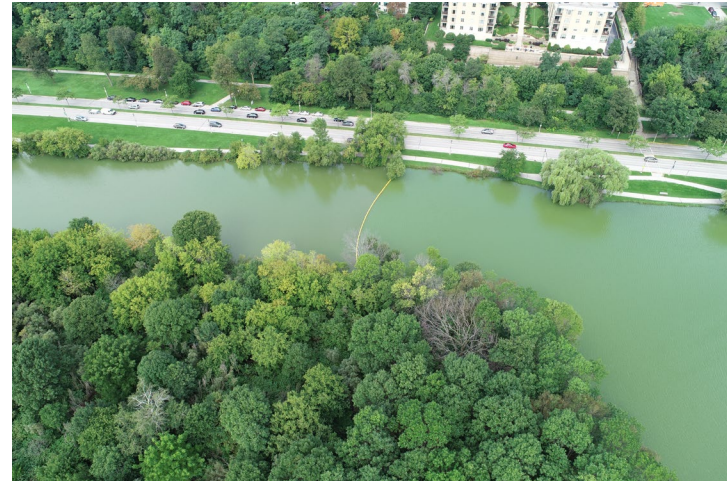
W – View of Turbidity Curtain
