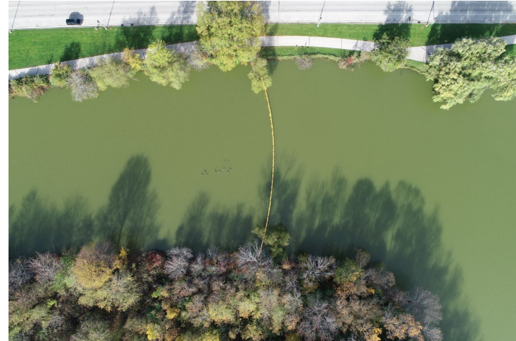
W – View of Turbidity Curtain
