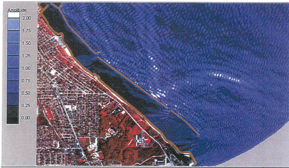
Figure A-19: Case 7 model output with 160 degree wave approach, 5m input wave-height and high SWE
