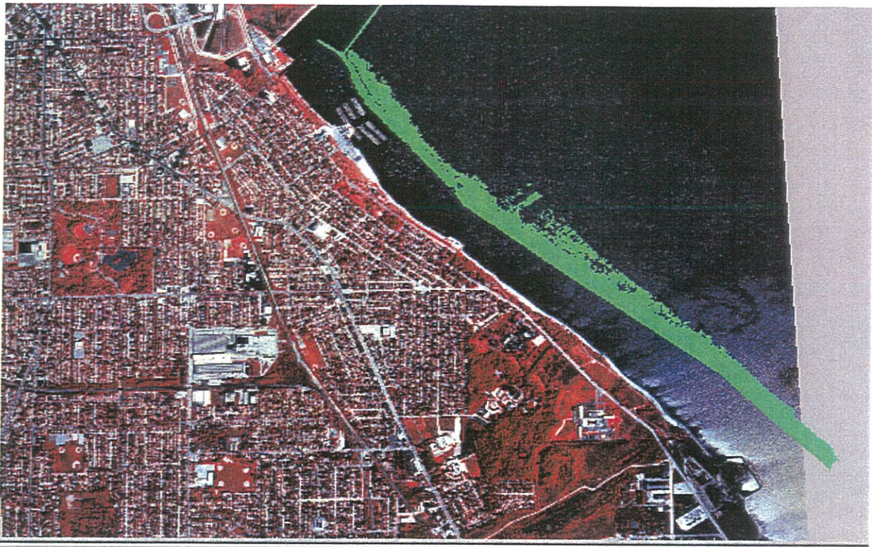
Figure A-2: Extent of SHOALS coverage during 1998 survey. Green zone represents acceptable SHOALS data.
