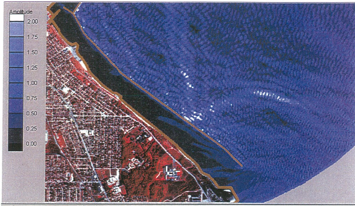
Figure A-23: Case 10 model output with 160 degree wave approach, 5m input wave-height and high SWE
