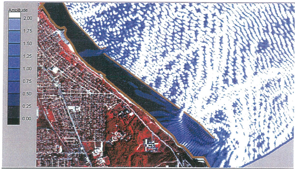
Figure A-17: Case 5 model output with 20 degree wave approach, 5m input wave-height and high SWE
