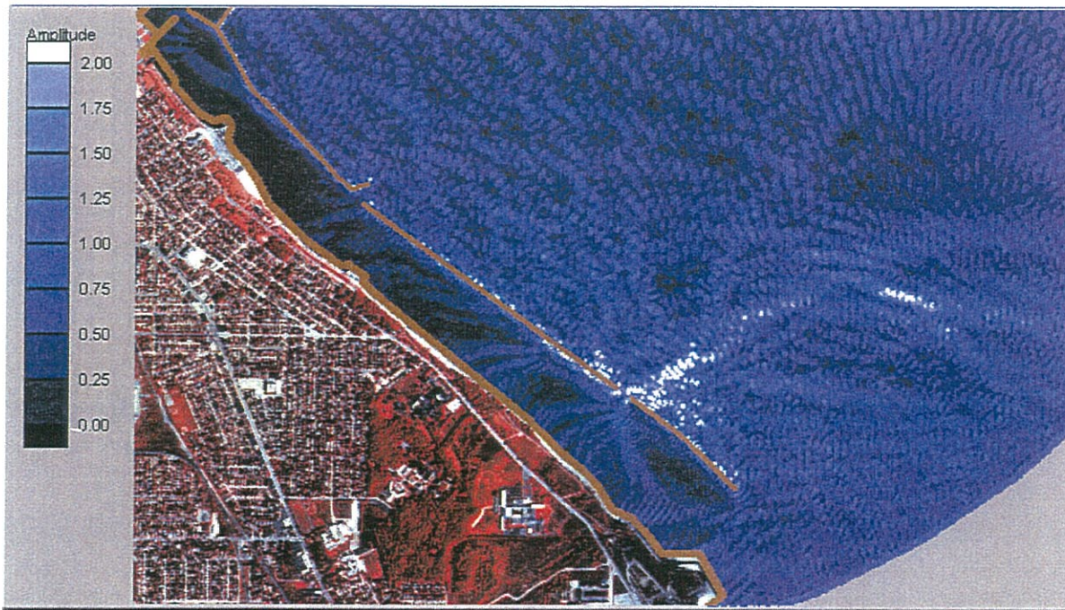
Figure A-16: Case 4 model output with 160 degree wave approach, 5m input wave-height and low SWE
