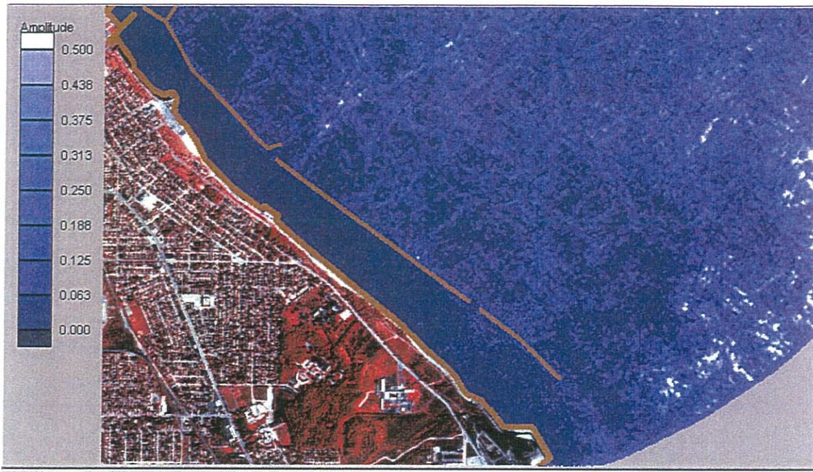
Figure A-15: Case 3 model output with 160 degree wave approach, 1m input wave-height and low SWE
